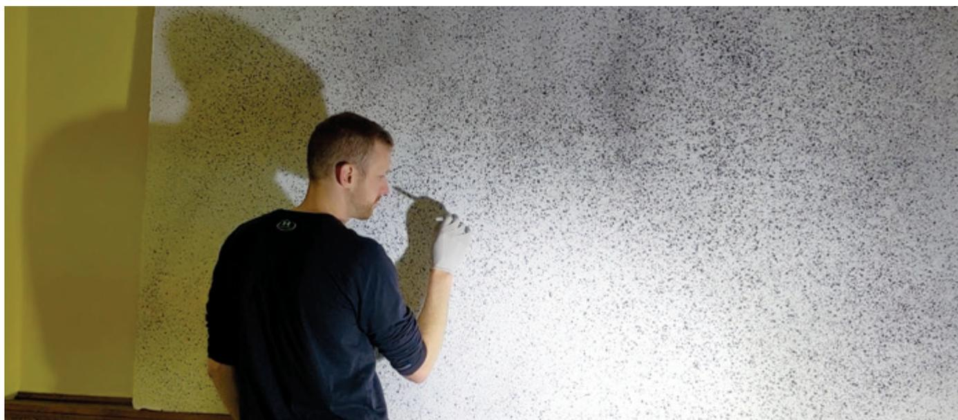
*A black marker is being used to make small dots in places on the drywall with relatively low speckle areal density. The image of these speckles by the camera are what become distorted by slight changes in the air, revealing the air flow that can be imaged using a high-speed camera.*
